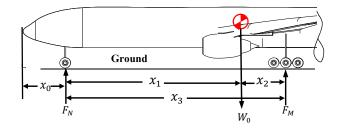
Fig. 9. Load distribution and various distances of a typical aircraft.
