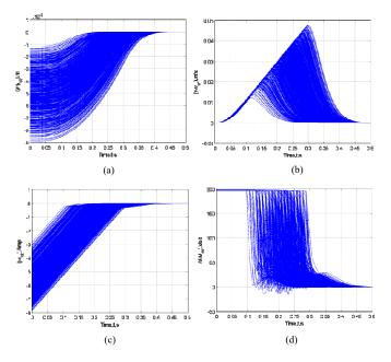
Figure 3 EMA residual profiles for 1000 Monte-Carlo trials; (a) ball position vs. time; (a) actuator position vs. time; (b) actuator velocity vs. time; (c) coil current vs. time; (d) coil voltage vs. time
