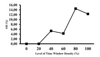
Fig. 4. Effect of time window density to the occupation rate of motorbike
