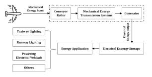
Fig. 7. Simplified block diagram of the proposed RPG model.
