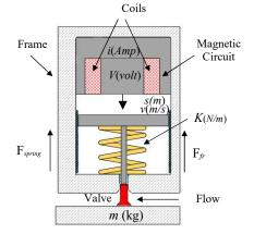
Figure 1 Electromagnetic Actuator Schematic
