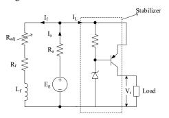
Fig. 10. Equivalent circuit diagram of the generator.
