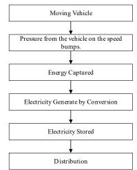
Fig. 1. General Principle of the RPG method.
