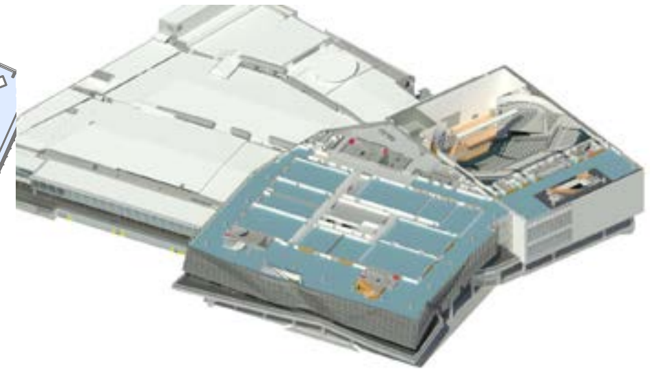
Axonometric cutaway view of Level 4 Convention Centre
